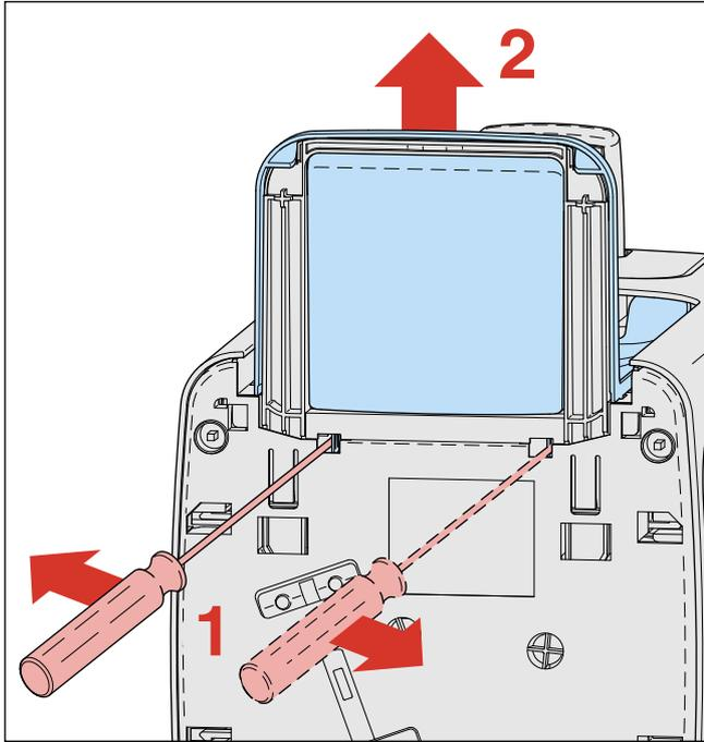
4. To remove the side panels unlock the 2 snap locks at each side and gently pull of the panels.
